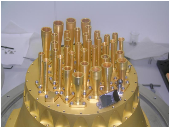
Left: corrugated feed horn array designed and manufactured for the High Frequency Instrument on Planck – ESA's cosmic microwave background surveyor. Right: a quasi-optical multiplexer separating 22, 43, 89 and 123 GHz bands, designed and built for the Korean VLBI astronomy Network.
