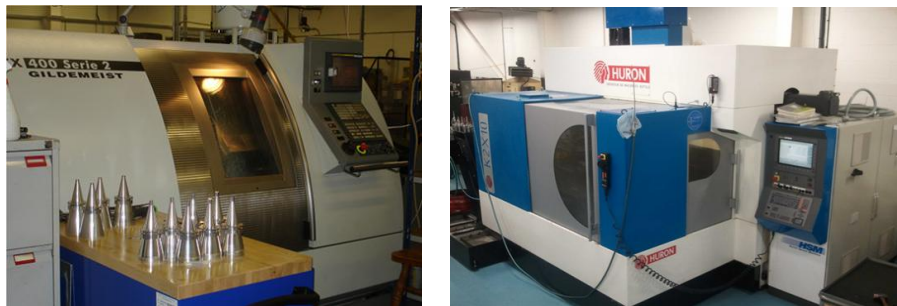
Clockwise from top-left: Thomas Keating Ltd. in West Sussex, Brown and Sharpe co-ordinate measuring machine in a temperature-controlled area, HURON high-speed milling machine and DMG Gildemeister lathe with a number of ALMA primary absorber structures.
