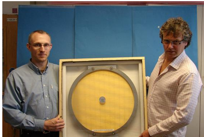
One of a pair of large wire grid polarisers, each using more than 3 km of wire.
