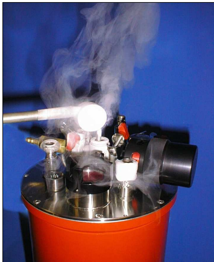
Photo 4.2. Helium gas exhaust during fill
