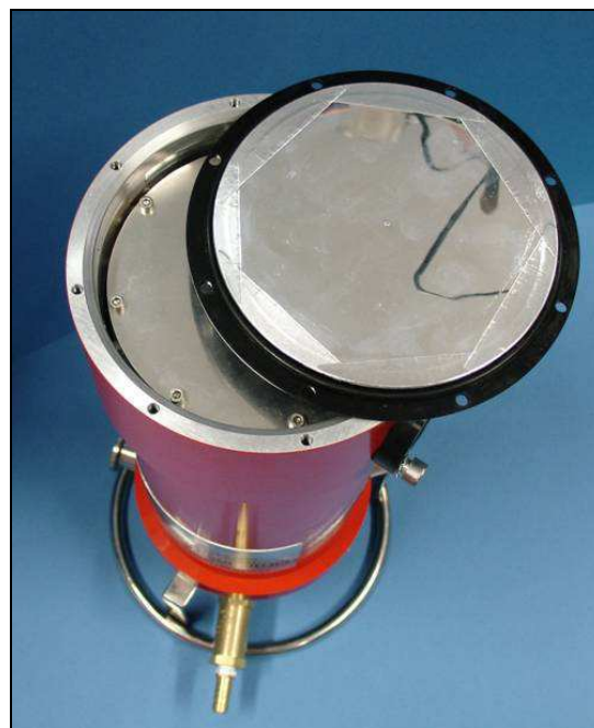
Photo 1.3. Radiation shield base-plate in position
