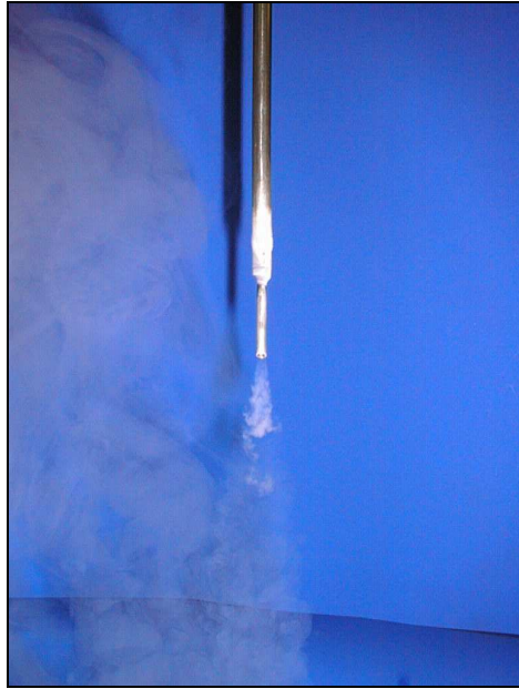
Photo 4.5. Liquid helium emerging from a cold tube
