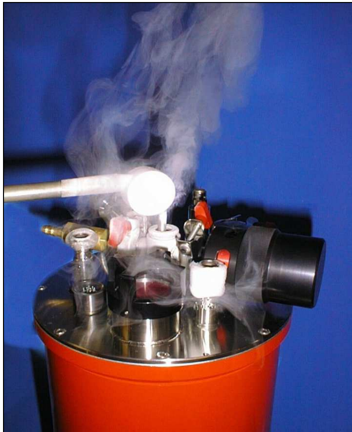
Photo 4.2. Helium gas exhaust during fill
