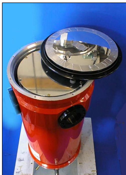
Photo 1.4. Liquid nitrogen base-plate in position
