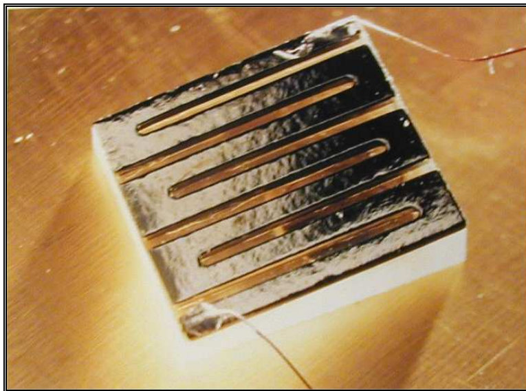
Photo A1.1. InSb detector manufactured as a toaster element mounted on a quartz substrate
