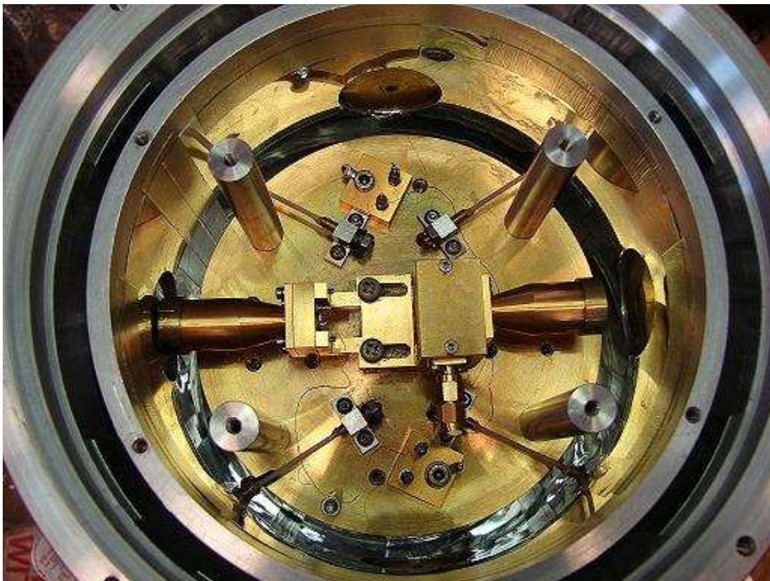
Photo 1.2. The four support pillars and the detector optics
